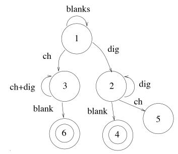
**These machines recognize** regular languages. To implement a finite-state transducer one begins with a GOTO table that defines transitions between states:
